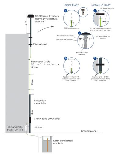
**IMPORTANT NOTE:** In installations with significant risk of receiving external induced surges (telecommunication towers, radars, substations, etc.), the FIBER mast will always be placed.
