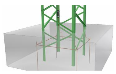
Figure 4. Installation of a dinfil filter on the DDCE downstream cable for its protection.
