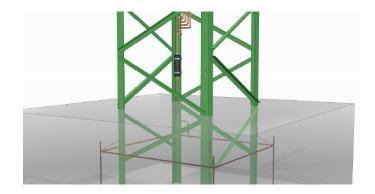
Figure 5. Dinfil filter type installation to protect the DDCE and all the electrical and electronic equipment of the tower (by means of an equipotential bar).
